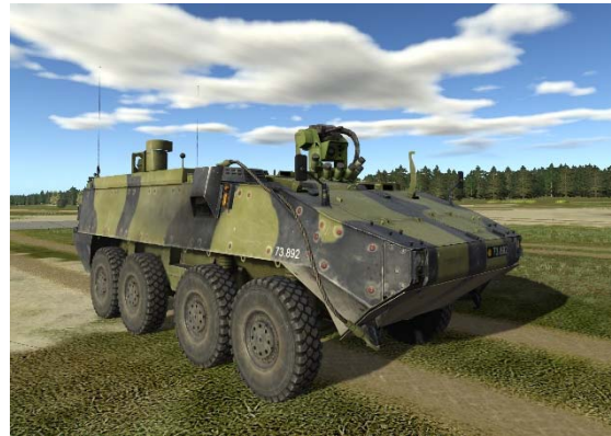
Piranha-IIIIC with Lemur RWS (40mm AGL configuration)
